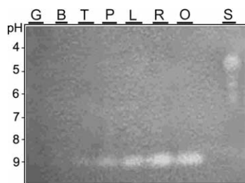
Fig. 2. Native PAGE IEF of tomato endo - \beta -mannanases resolved on a broad range pH 3–10 gel and visualised using an azo-galactomannan overlay. Equal amounts of crude protein extract were loaded in each lane from ripening fruit (G, mature green; B, breaker; T, turning; P, pink; L, light red; R, red; O, overripe) and 4-day-old seedlings (S).
